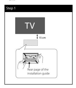
When you mount on a wall(concrete), use the wall plugs and screws (Not supplied). Attach the wall bracket on the wall as shown in the illustration below.
